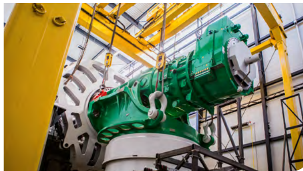
Tests conducted in the Fraunhofer Dynamic Nacelle Testing Laboratory simulate rotor stress and grid fluctuations. © Adwen
