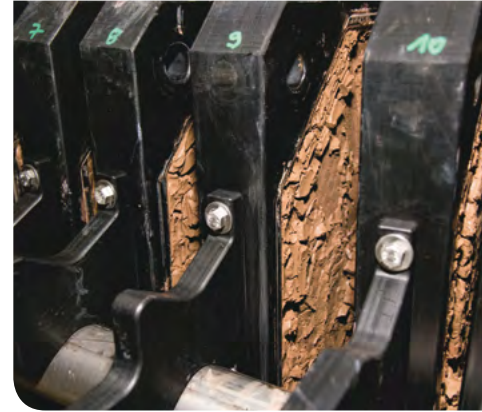
From left to right: Filtered lignin after precipitation from a digestion solution.
