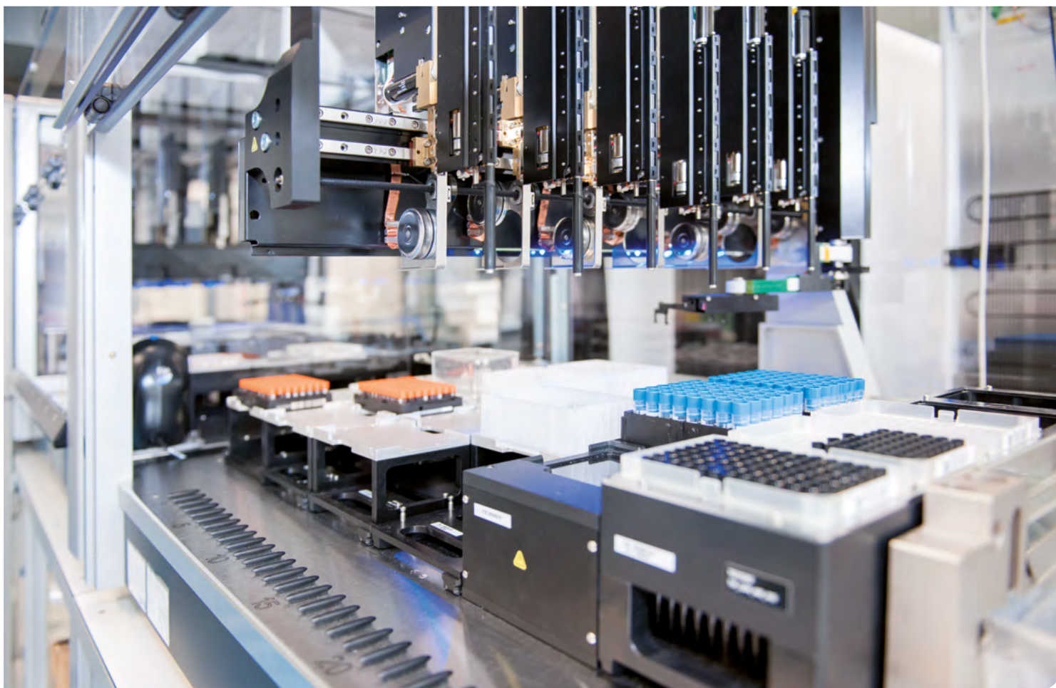
Fraunhofer IZI's pipetting robots isolate RNA from tissue samples in search of new biomarkers to diagnose prostate cancer. © Fraunhofer IZI
