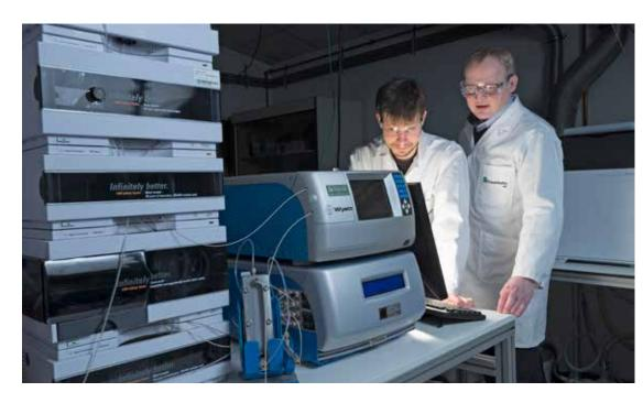
Boris Meisterjahn and Prof. Dr. Christian Schlechtriem in the laboratory with the AF4 system (used to fractionate nanoparticles). Fraunhofer IME offers state-of-the-art techniques for the characterization of nanomaterials.
