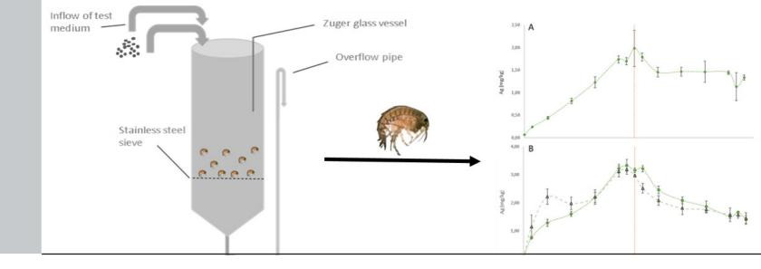
Overview of the flow-through system to test nanomaterials.
