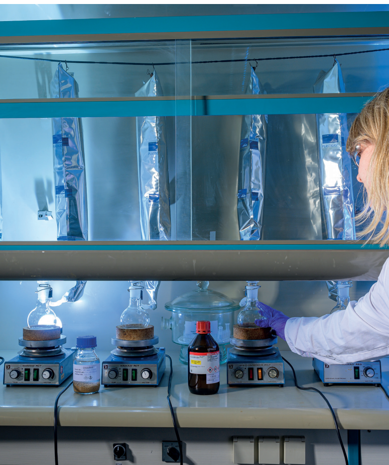
Laboratory set-up for the determination of NER Type I (Silylation). Photo: © Fraunhofer IME | Klaus-Peter Kappest
