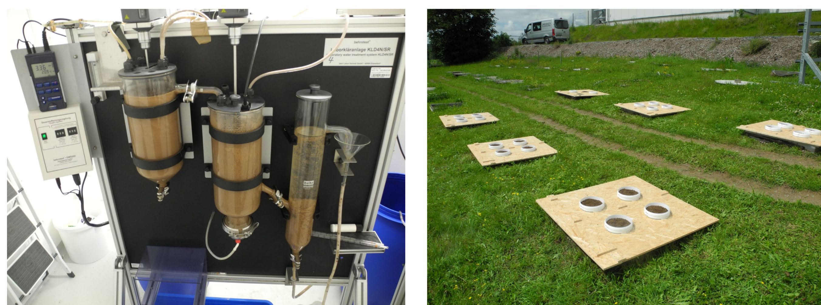
Figure 1: Test performance on fate and effect of MPs using a model sewage treatment plant (left picture) followed by an outdoor lysimeter experiment with soil-sludge mixtures (right picture).
